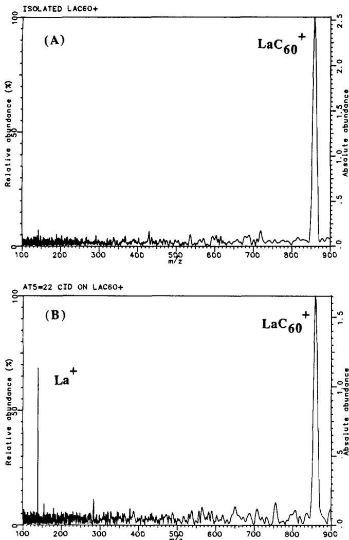
**Figure 1.** Plot of relative abundance vs  $m/z$ : (A) isolated  $\text{LaC}_{60}^+$ ; (B) collision-induced dissociation of  $\text{LaC}_{60}^+$  (105 eV Laboratory, 4.7 eV center of mass energy) yielding  $\text{La}^+$ .
