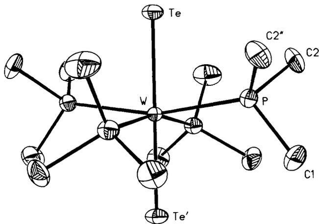
**Figure 1.** ORTEP drawing of  $trans-W(PMe_3)_4(Te)_2$ . Selected bond lengths (Å) and angles (deg): W–Te = 2.596 (1), W–P = 2.508 (2); Te–W–Te' = 180.0, Te–W–P = 82.1 (1), Te'–W–P = 97.9 (1), P–W–P\* = 91.1 (1), 164.2 (1) (an asterisk indicates other phosphorus atoms).
